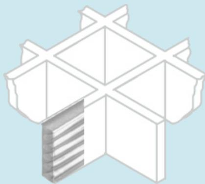
Molded grating is made by layering liquid resin and long continuous fiberglass strands inside an open mold.
